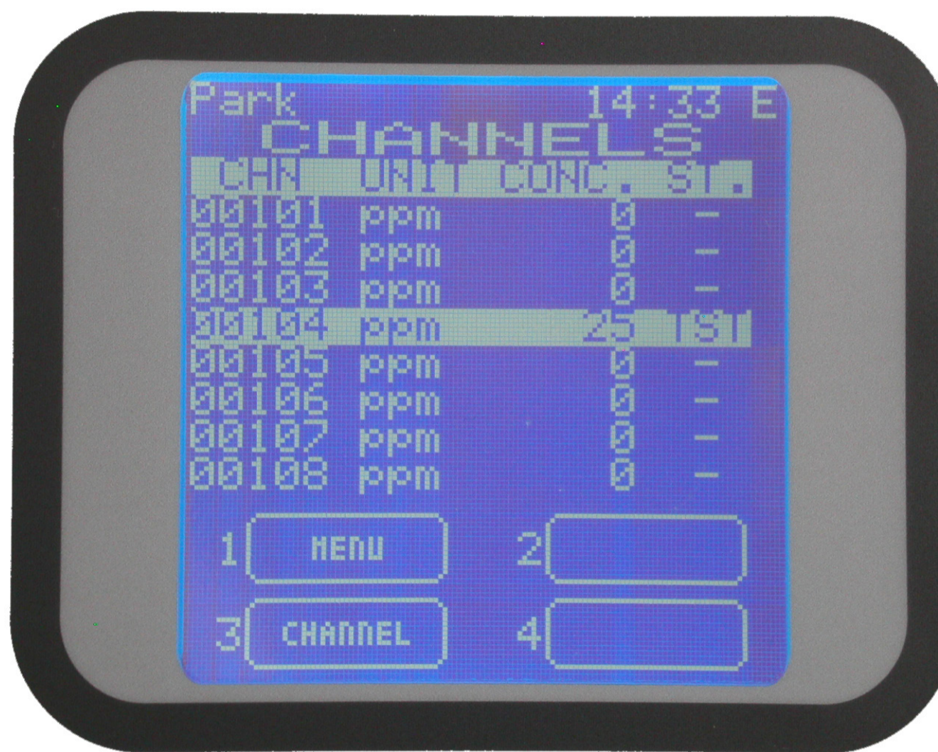
Figure 43 Screen with channel in "Test"
