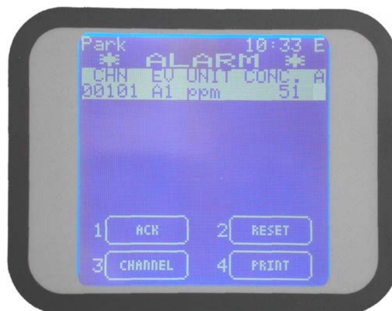
Figure 22 Typical ALARM state of the ACTIVE EVENTS screen.
