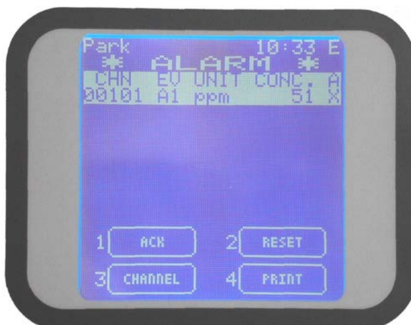
Figure 28 Active Events screen with alarm only
