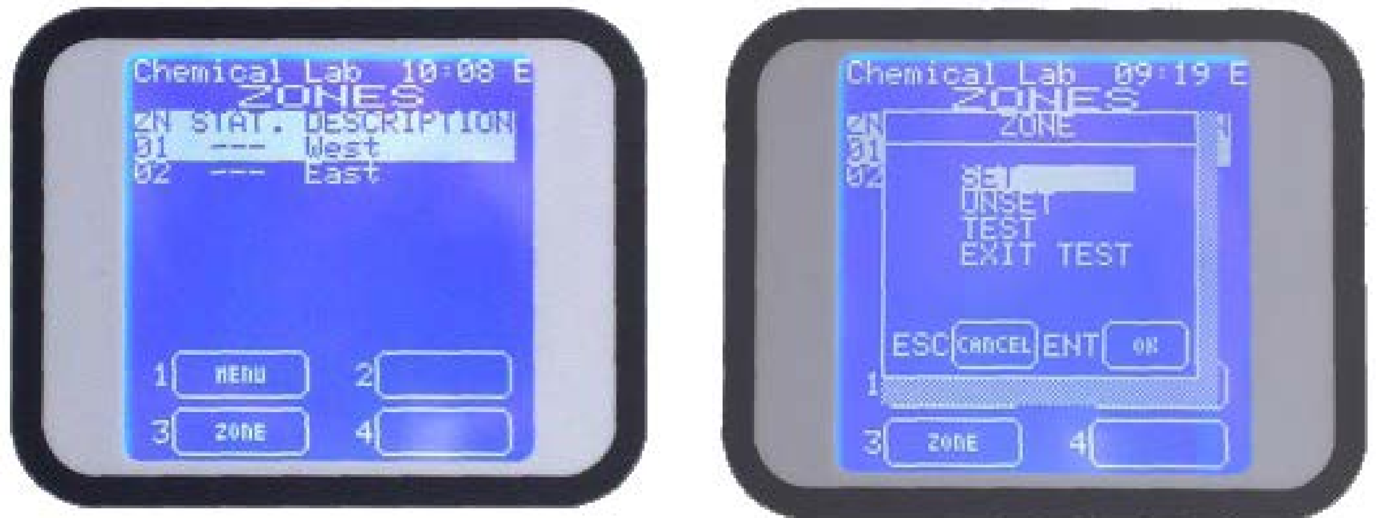
Figure 36 Zones screen and available options pressing 3-Zone
