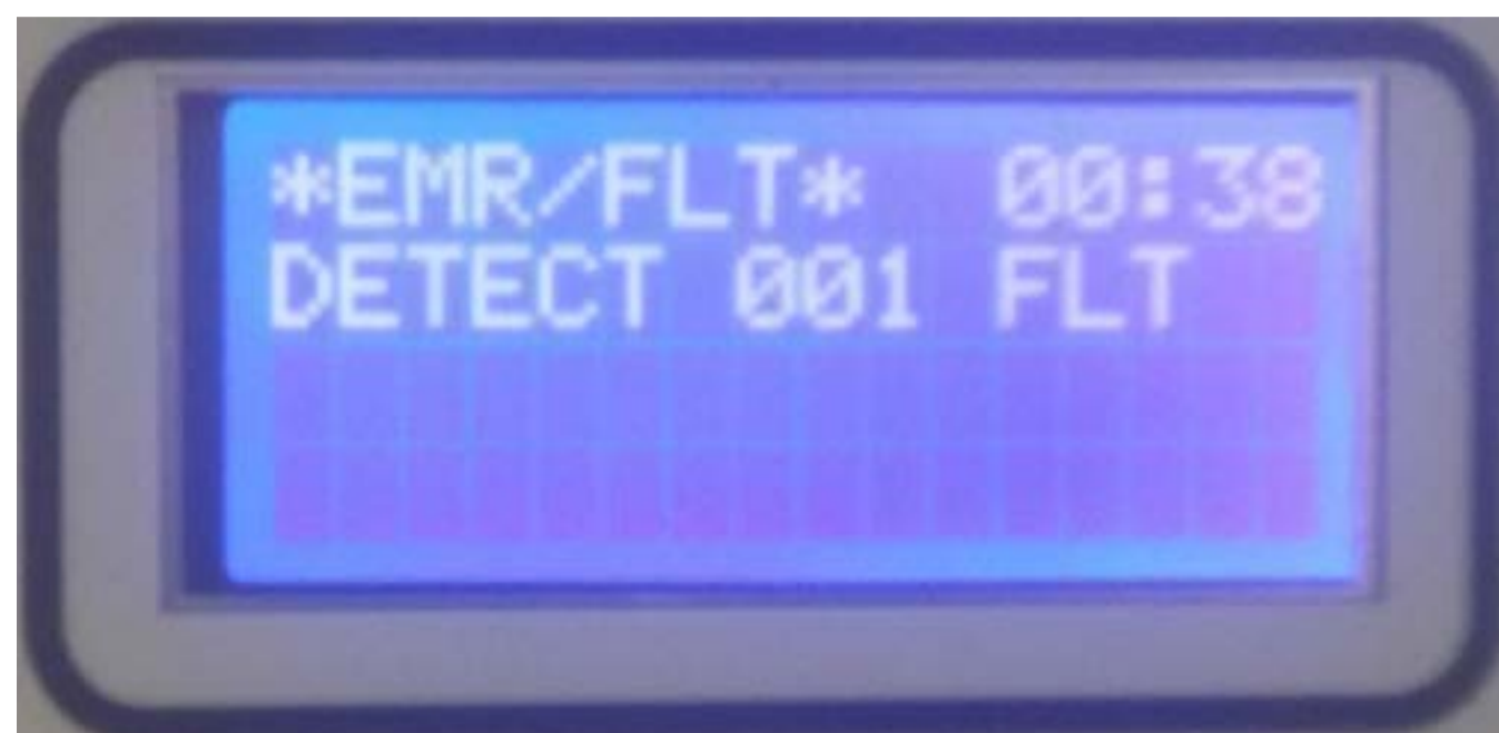
Figure 25 Typical FAULT state screen.
